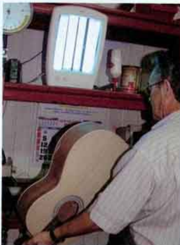
In one of Alhambra's numerous quality-control stages, special fluorescent lights are used to expose minute spots of excess glue prior to the finishing process.
